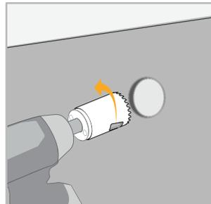
When cutting a circular hole use a hole saw, and run it backwards to minimize pulling.
