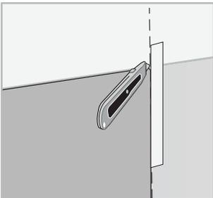
Trim panels along the end to fit using a straight edge and cutting tool.
