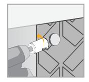
When cutting a circular hole use a hole saw, and run it backwards to minimize pulling.
