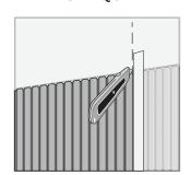
Trim panels along the end to fit using a straight edge and cutting tool.
