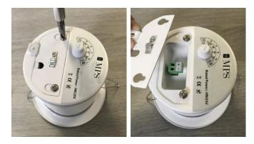
2) Pass the power wire(s) through the wire guide lock and connect the wires in the green terminal block.
