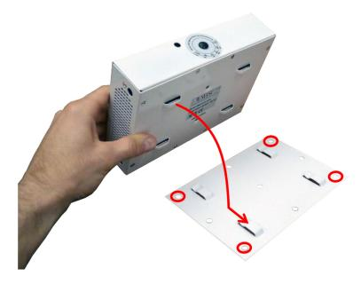
Note: When mounting the speaker on a vertical surface, be sure to mount the bracket with the forks facing up to avoid the speaker from falling down.
