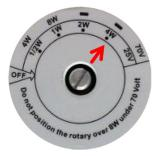
The recommended tap for most applications is 4W @ 25V. Some limitations may apply to the sound masking controller. See controller specifications for more details.
