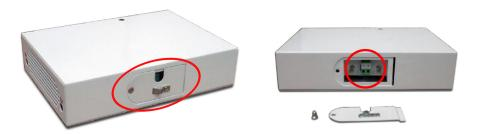
2) Remove the connector block, connect the wires and put back the connector block in place. Use plenum rated cable and follow local regulations. Typical wire will be 18/2 FT4.
